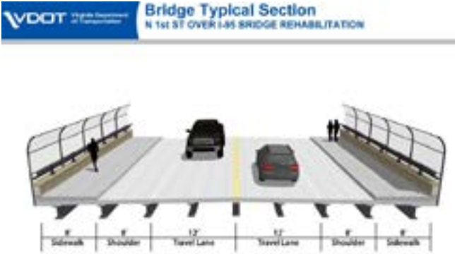
Typical Bridge Section Created by VDOT
