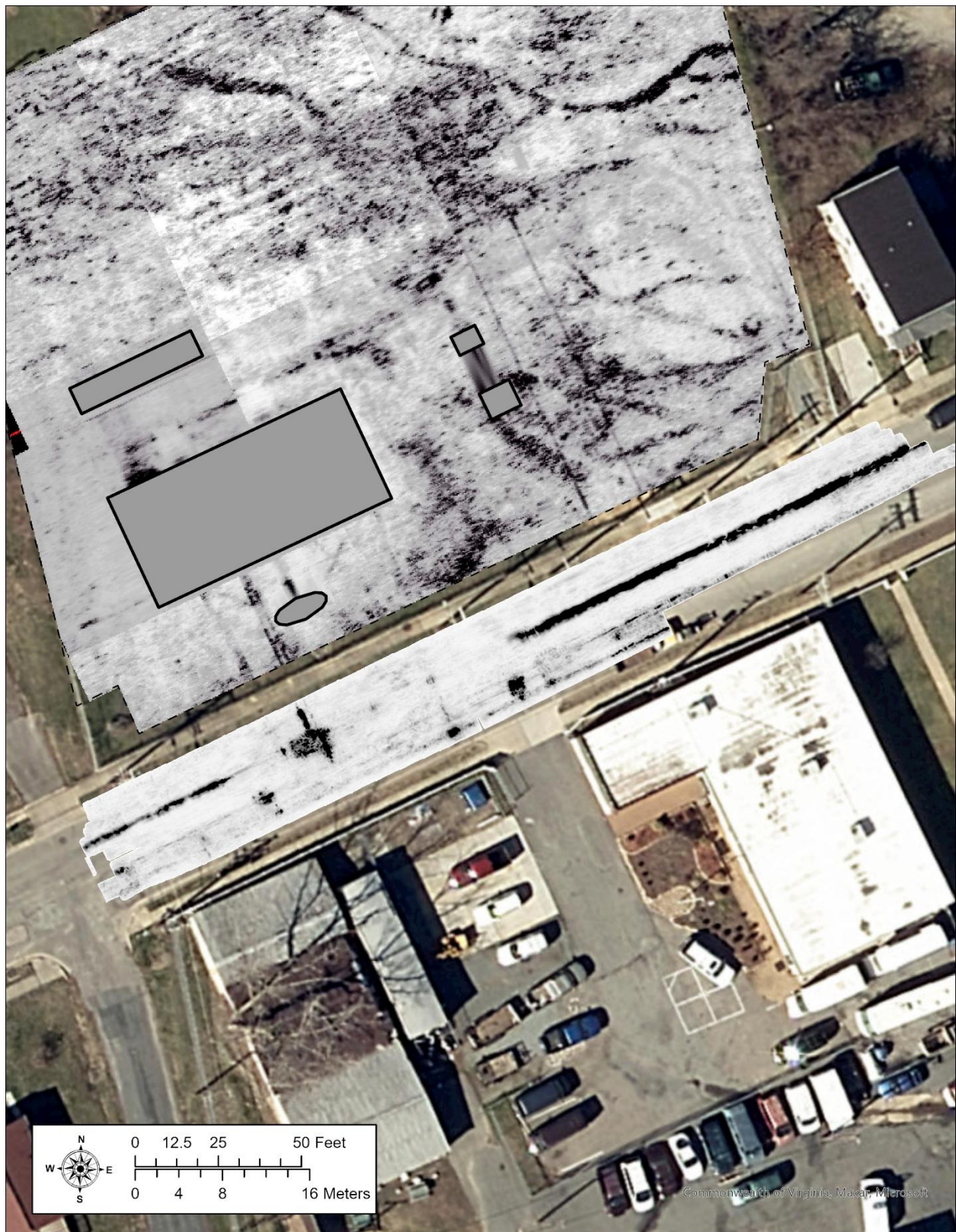
Figure 5.14. MALA HDR GPR interpolation map of utilities beneath Wise Street (2 ft interval slice).
