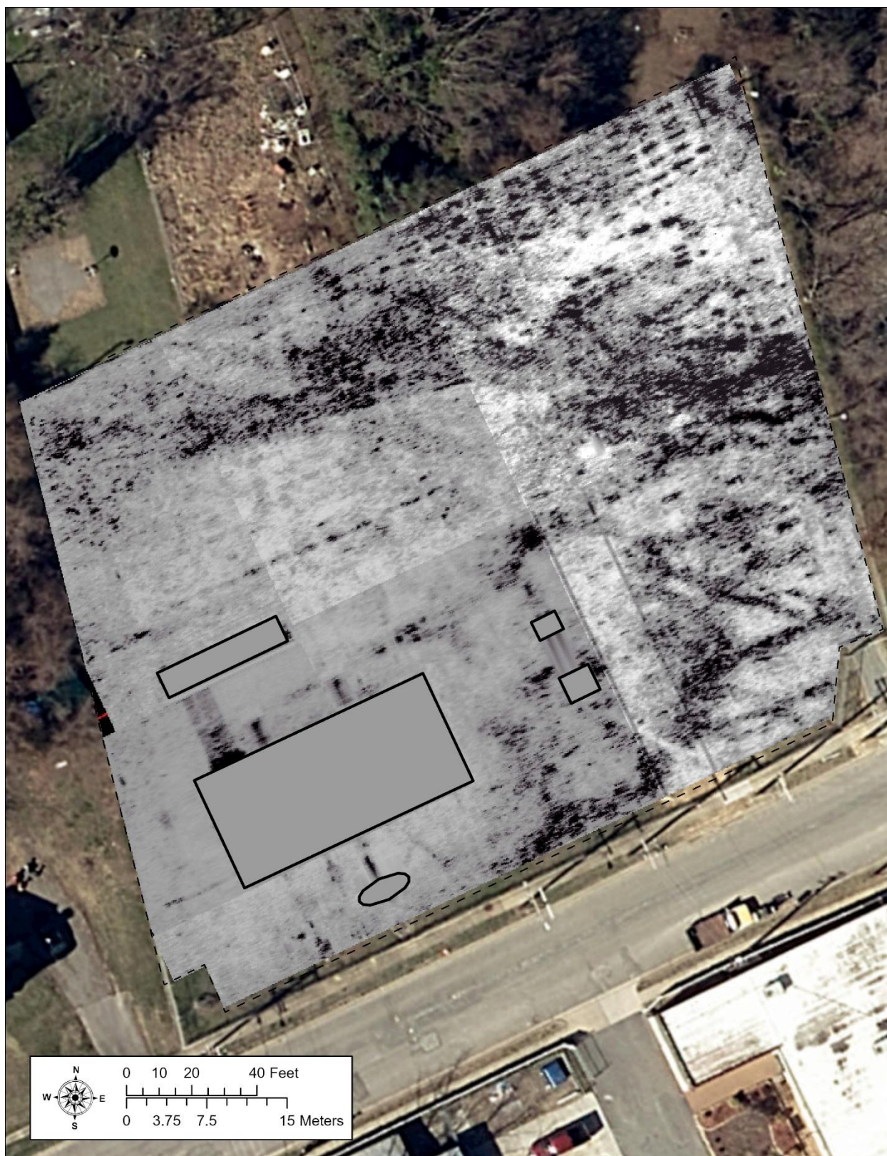
Figure 5.10. Three-dimensional interpolation map of potential burials at the 1857 Manchester Municipal Cemetery at 3.50 ftbs (1 ft slice thickness), non-annotated.
