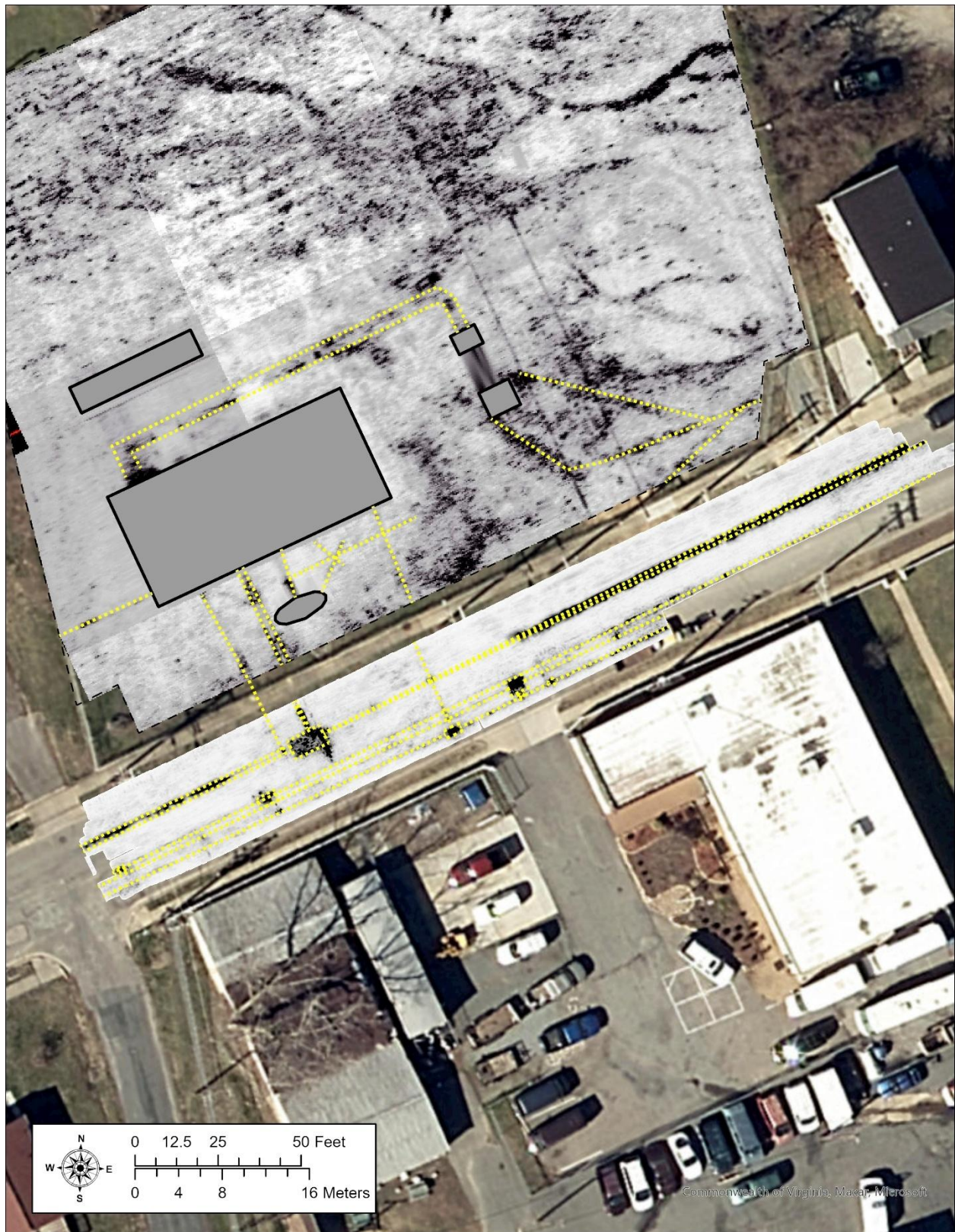
Figure 5.15. Annotated MALA HDR GPR interpolation map of utilities (dotted yellow lines) beneath Wise Street (2 ft interval slice).
