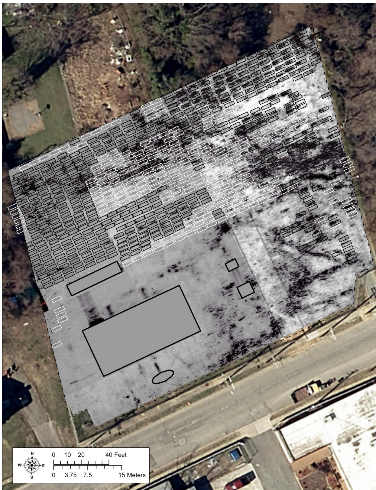
Figure 5.11. Annotated three-dimensional interpolation map of potential burials at the 1857 Manchester Municipal Cemetery at 3.50 ftbs (1 ft slice thickness) showing probable graves (black outline) and possible interments (white outline).
