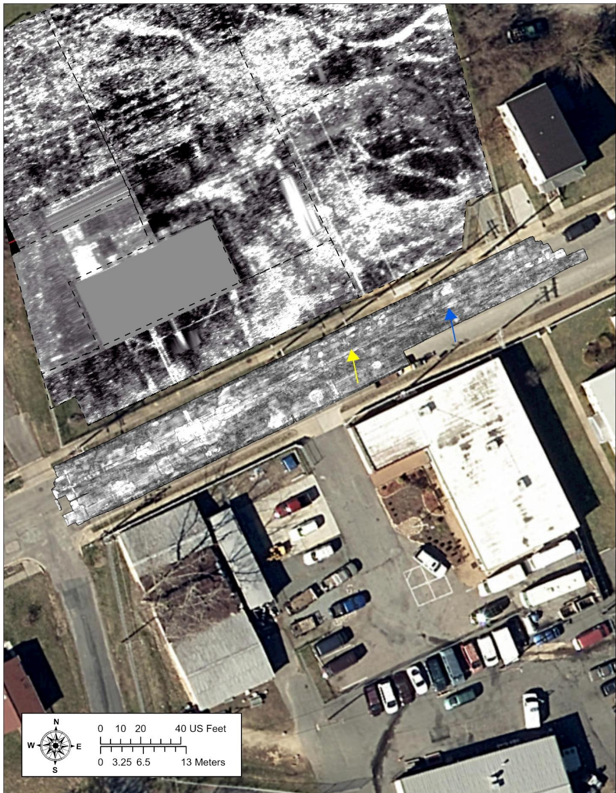
Figure 5.12. MALA HDR GPR interpolation map of potential burials in Wise Street (yellow and blue arrows).
