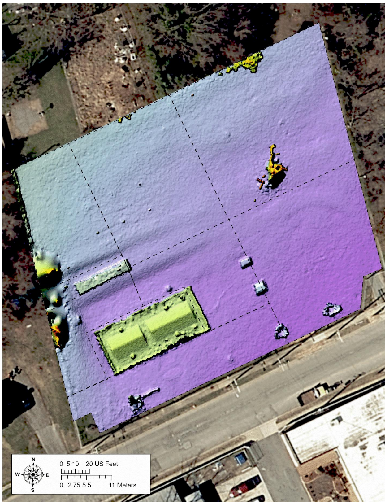
Figure 5.8. DEM of the 1857 Manchester Municipal Cemetery derived from drone imagery. Note the exceptionally faint rows of potential subsided graves shafts in the northern half of the DEM.
