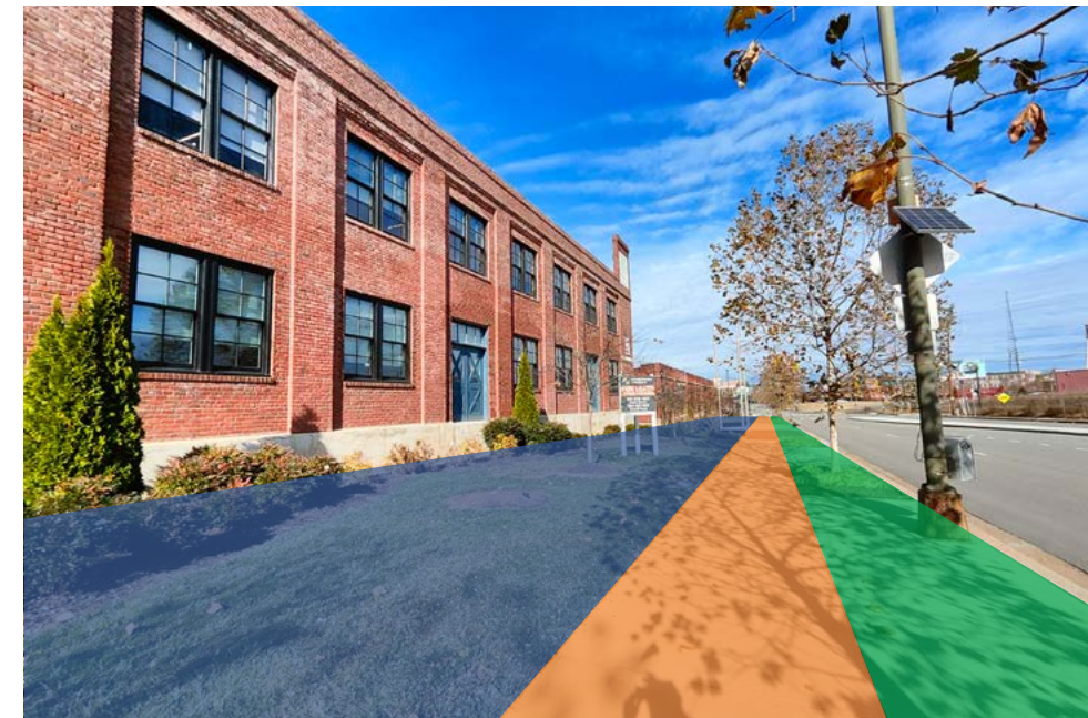
A clear delineation between the Frontage Zone (blue), Pedestrian Travel Zone (orange) and Buffer Zone (green).
