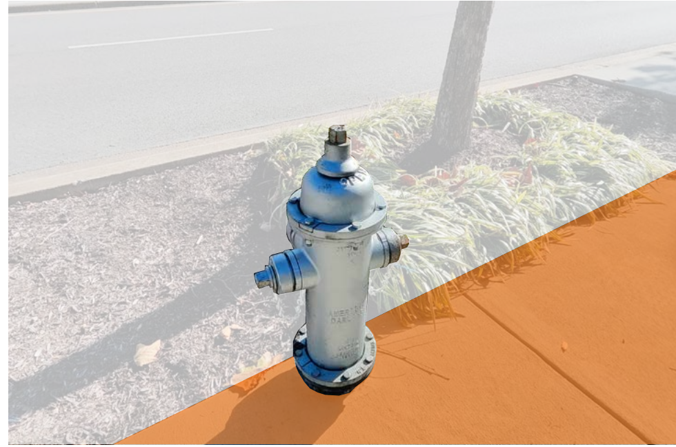
Fire hydrants on site are located within the Pedestrian Travel Zone (orange), reducing the width of the walkway for pedestrians.
