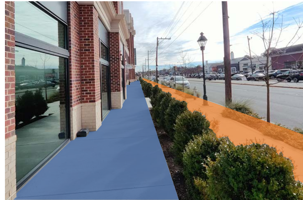
Frontage Zones and the Pedestrian Travel Zones are clearly distinguished through an evergreen hedgerow and elevation change.
