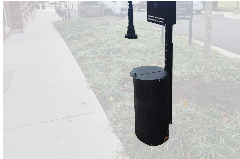
Pet waste stations, light poles and wayfinding signs are located within planting beds to avoid obstacles in the Pedestrian Travel Zone.
