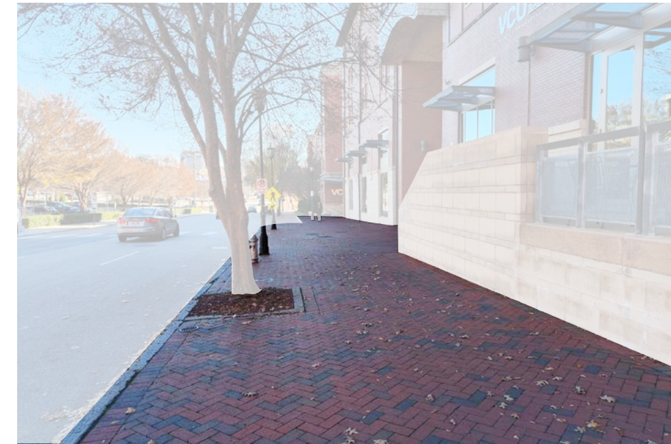
A wide pedestrian sidewalk with smaller tree wells are suitable for larger volumes of pedestrian traffic.
