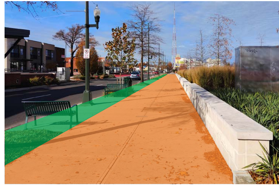
The Pedestrian Travel Zone (orange) is clearly distinguished by the street furnishings located inside the Buffer Zone (green) and a lack of obstructions in the walkway.
