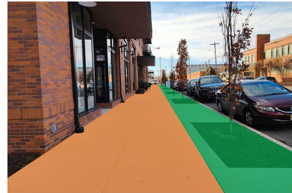
A clear delineation between the Pedestrian Travel Zone and the Buffer Zone however, the Frontage Zone is not clearly marked.
