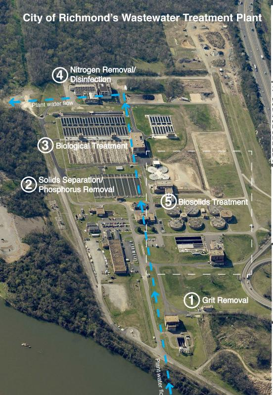
1 In this preliminary treatment stage, wastewater flows to the headworks by gravity. Grit, rags, and heavy debris are removed and taken to a landfill off-site. Water is pumped from the lift station to the primary clarifiers.
