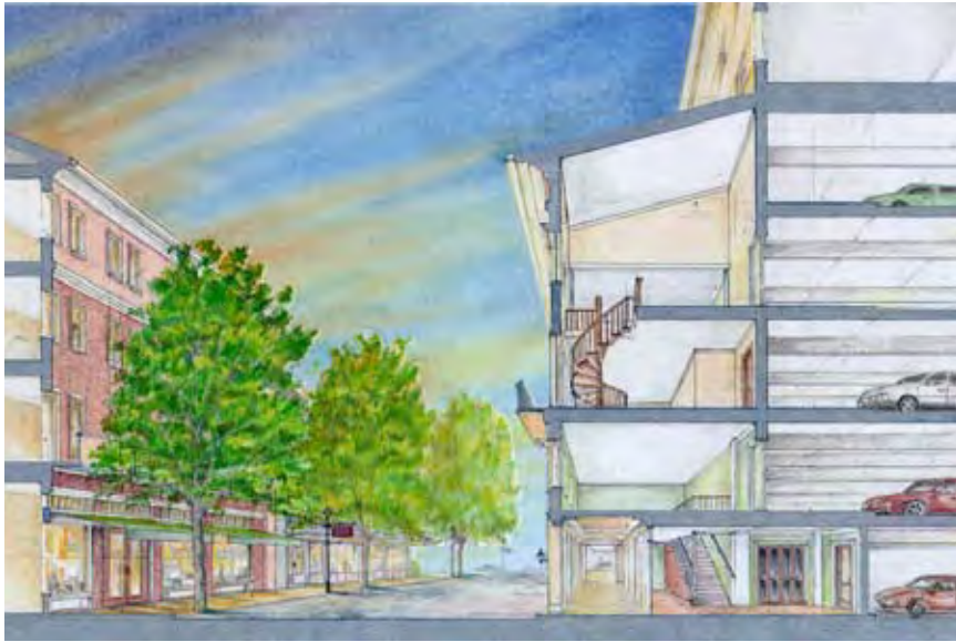
This cross-section demonstrates a liner building that masks a mid-block parking garage, allowing off-street parking to be integrated into a pedestrian-oriented neighborhood.-
