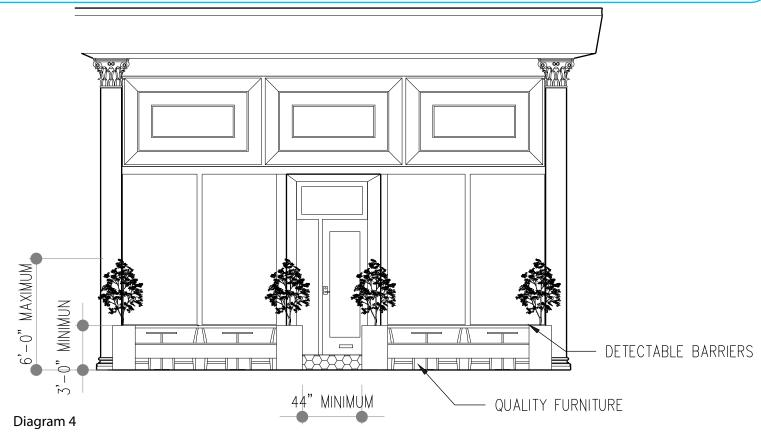
Elevation view of a sidewalk café showing café elements and access opening.
