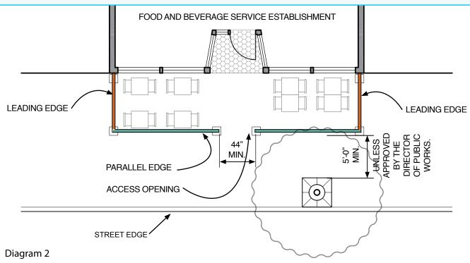
Plan view of a sidewalk café that extends more than 3 feet or more into the sidewalk.
